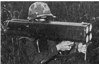
Being tested in late 1971 is the MX191 flame weapon, which can fire a four-round clip of rockets equipped with incendiary warheads at the rate of about one per second.
